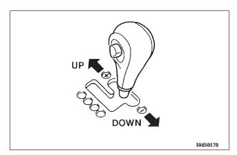
+ (UP): Push the lever forward once to shift up one gear.- (DOWN): Pull the lever backward once to shift down one gear.
